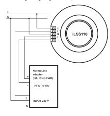
Please note Once the fitting is connected to mains and it is turned off, the relay will remain closed and the - + output will be at maximum while the stabilization takes place (aproximately 1 minute).
